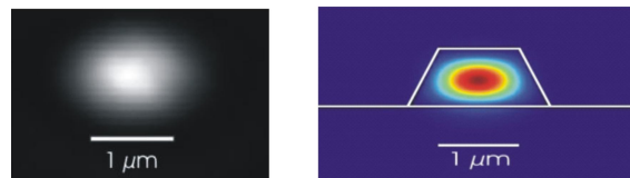
Fig. 4. Measured (left) and calculated (right) intensity distribution of the fundamental mode in a LNOI channel waveguide of 1 \mu\text{m} top width (qTM-polarization; \lambda = 1.55 \mu\text{m} ). The profile, used for the simulations, is indicated (right).
