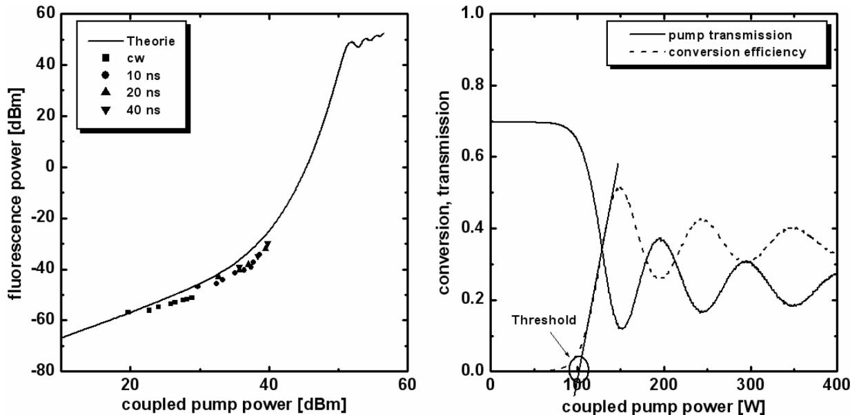
**Fig. 1:** (left) Calculated and measured fluorescence power ( $\lambda_s = 3400$  nm,  $\lambda_i = 2849$  nm) versus coupled pump power ( $\lambda_p = 1550$  nm). (right) Pump transmission and conversion efficiency as a function of coupled pump power at the same operating point.
