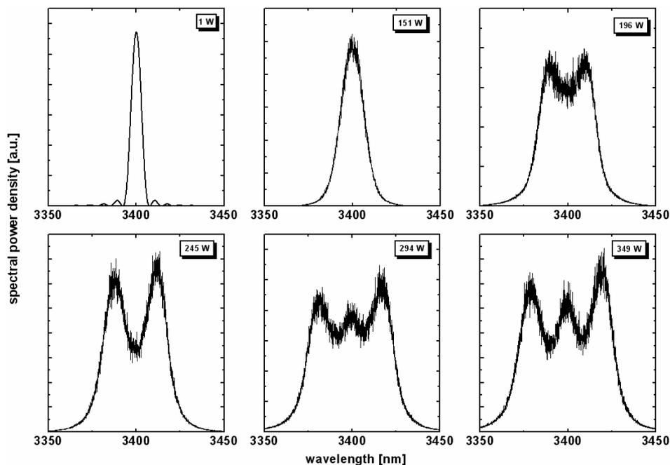
**Fig. 3:** Fluorescence spectra for different pump levels in arbitrary units of spectral power density.
