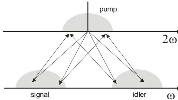
Fig. 2: Mechanism of incoherent nonlinear broadening.
